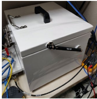
Figure 48. The commercial Faraday cage used in the experiment
